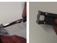
Cut and remove the cover for the cables on the back (possibly with a screwdriver push on template to facilitate the cutting).
