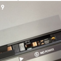
Slide the terminal inside the body of the Power Track until snap the clip system and replace the silicon rubbers.
