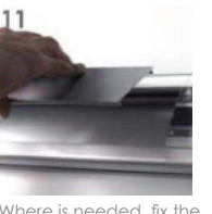
Where is needed, fix the blank cover (aluminum cap) in the profile.
